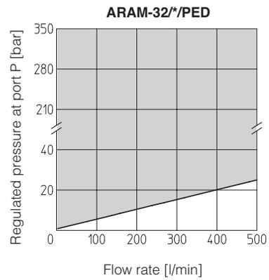
**11 MINIMUM PRESSURE VERSUS FLOW DIAGRAMS** based on mineral oil ISO VG 46 at 50°C
